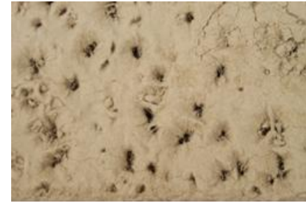
Flat Sheet Dust Loading Nonwoven Depth Type Media 200 cm/s, ISO Fine
