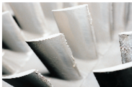
Fig. 2: Dust encrustations on rotor blades in an industrial gas turbine (6 MW)
