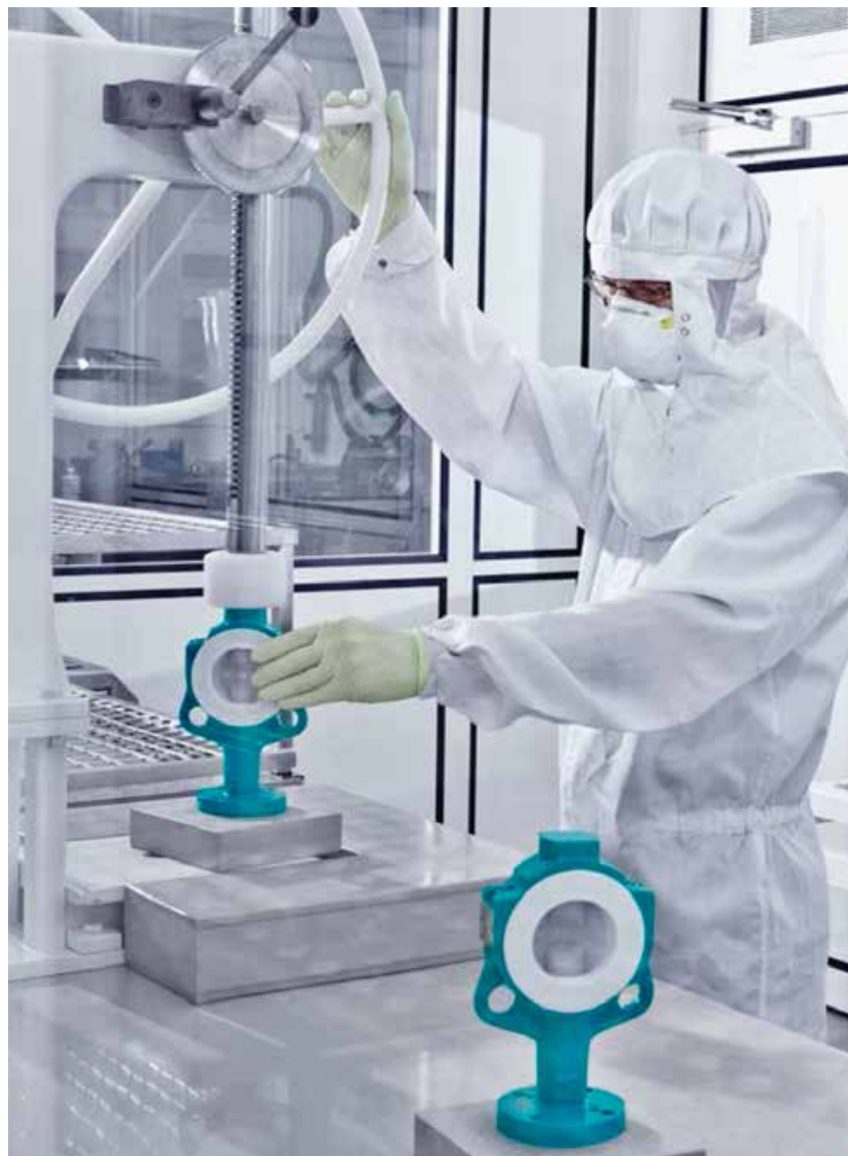
Assembly of the Bianca butterfly valve in the clean room. Image credit: https://www.interapp.net/downloads/casestudies/IAP_CaseStudy_Ovivo_1823en.pdf .
